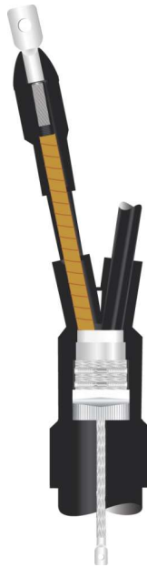
1.1 kV PILC Termination
